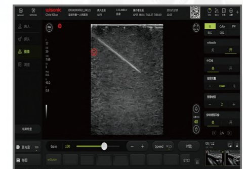
Auto Needle Enhancement, auto needle detection, and auto acoustic beam adjustment
