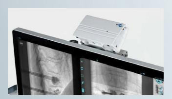
Optional Wi-Fi video transmission for high resolution, remote image display on wireless display unit, ceiling suspension or wall-mounted monitors.
