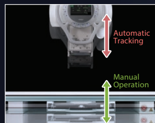
Motorized Vertical Synchronization with table, maintains constant SID
